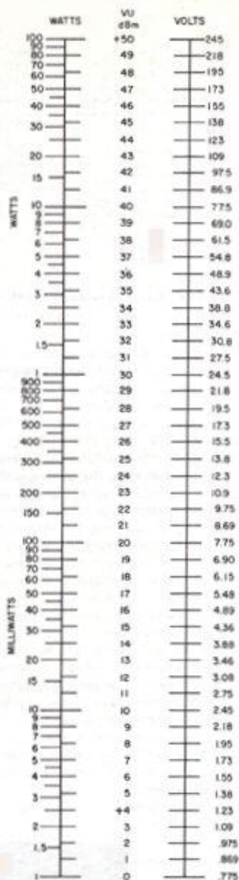
Fig. 10-42. Relationship of VU and dBm to power in watts and voltage in a 600-ohm line.
